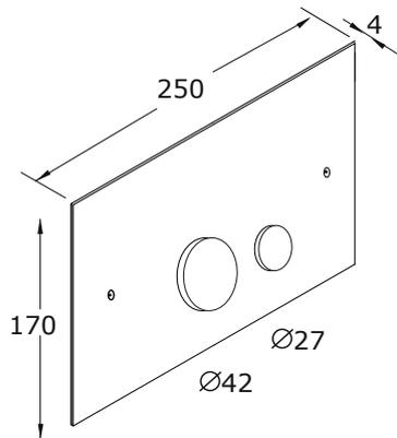
Suitable on flush tanks Geberit Italia UP720 and UP320 produced from 2010
